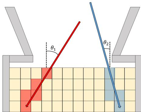
Figure 4: This diagram shows how different arrays are illuminated by an incident electron. For a given illuminated arrays, the onboard computer can compute what the probable incident pitch angle was. Also, as each detector will deplete some energy,  $\Delta E_{layer}$ , how far the electron penetrates into the stack gives an indication of what the total energy of the incident electron was.
