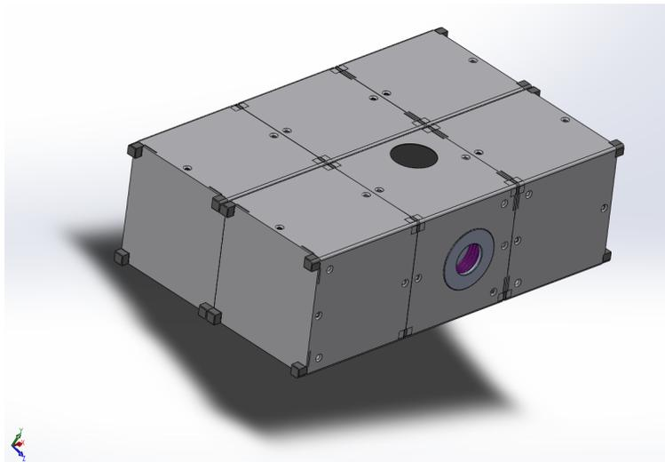
Figure 5: Image showing the detector port and star tracker port on the aft side of the spacecraft. Antennas and solar panels not shown.
