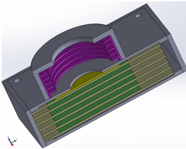
Figure 2: Shown is the design for the REPTAR detectors. The collimator is lined with Tungsten baffling, shown in purple, then after the field stop is a Be window to facilitate unwanted particle blocking, and finally the six silicon detectors
