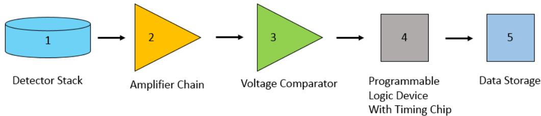
Figure 3: Shown is the flow of the backend electronics consisting of: detector stack, amplifier chain, comparator for discriminating voltage pulses, programmable logic device for binning the signals, and then on-board data storage and further processing if needed.
