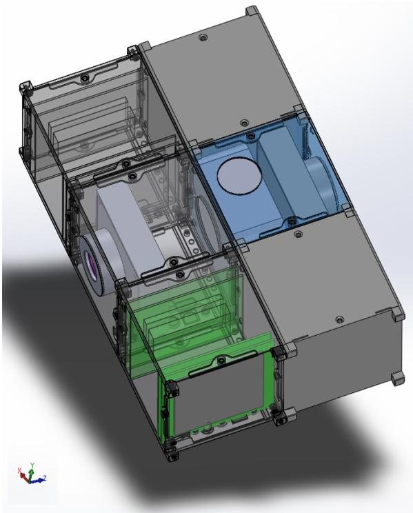
Figure 6: Image showing the boards for the space craft and the detectors back end electronics. Also shown is the ACDS system with port for star tracker, and the two detector assemblies. Antennas and solar panels not shown.
