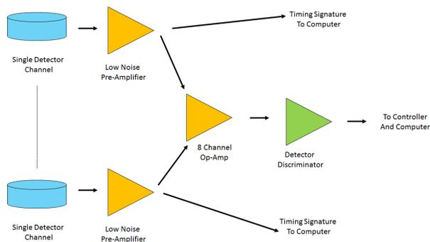
Figure 7: Figure showing back end electronics and how each channel will have its own low noise preamplifier, but will share a common high gain op amp with seven other channels. This signal is then fed into the discriminators and then to the onboard computer.
